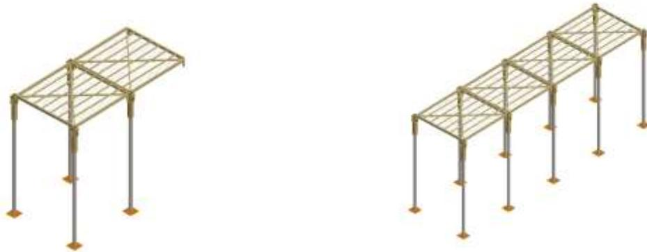
7. If the geometry dictates a gap in the centre of the run (see Step 8), lay an infill panel or deck panel over the gap and secure.
