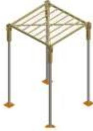
6. Carry on adding decks and tube legs with DUAL brackets on and erect and follow down the wall.
