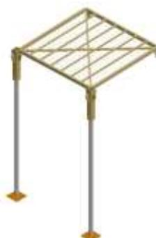
5. Then add an additional two tubes with DUAL brackets fitted to form the first m2.
